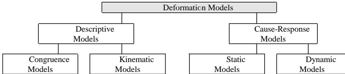
**Figure 3** Hierarchy of models in geodetic deformation analysis (Heunecke 1995, Welsch 1996)
