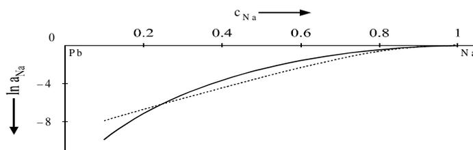
**Figure-2:** Activity ( $\ln a_{\text{Na}}$ ) of sodium in the sodium-lead liquid alloy at 700 K. for different concentrations of Na. The full curve represents the theoretical values. The dotted curve shows the experimental values due to Hultgren *et al* (1973).
