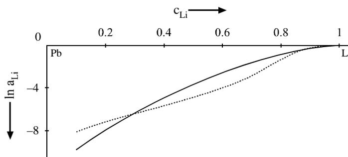
**Figure-1:** Activity ( $\ln a_{Li}$ ) of lithium in the lithium-lead liquid alloy at 932 K. for different concentrations of Li. The full curve represents the theoretical values. The dotted curve shows the experimental values due to Saboungi *et al* (1978).
