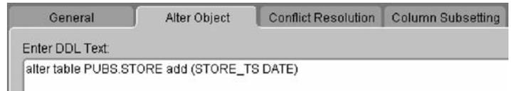
Figure 1. OEM Adding a Column to the store table
