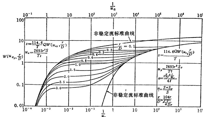
Figure 2. A portion of a page from the translation of Prickett (1965) in the book by Zhang showing Boulton's (1963) type curves for transient analysis of pumping in an unconfined aquifer.
