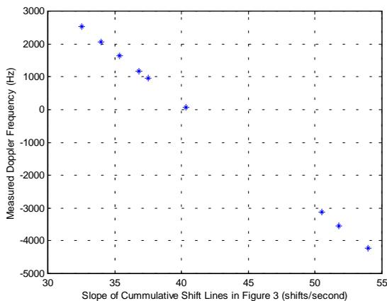
**Figure 4 – Doppler Frequency vs. C/A Code shifts/second**
